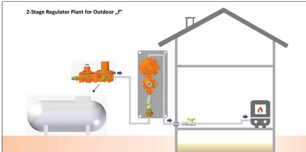
**A medium pressure 1st stage regulator, mounted directly onto the LPG tank. A low pressure 2nd stage regulator with main shut-off device in the house connection box for outdoor systems „f“ - optionally this can be mounted with a gas flow monitor “GS”.**
